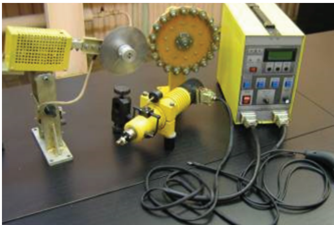
Low-voltage high-frequency equipment for PED
